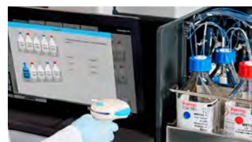
On-board management of bar-coded reagents and consumables with full traceability
